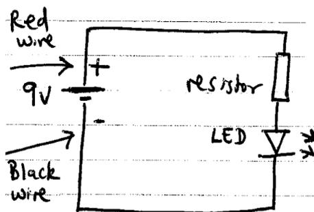
(The red and black wires are the wires of the 9v battery connector).
