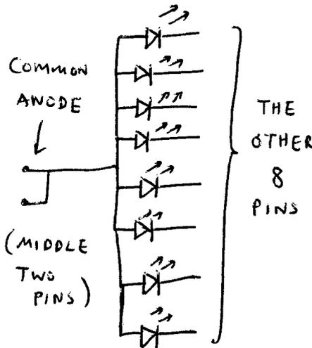
So how can you light up one of the segments? You connect the common anodes to the battery's positive terminal and then connect one of the other 8 pins to the battery's negative terminal via a resistor:
