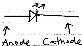
The LED will only work if the anode is more positive than the cathode and here's a circuit we could build that would work:
