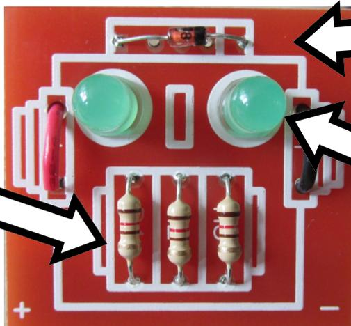
2. Solder the diode across the top 5 holes. IMPORTANT: the end with the black band must be on the right hand side.
