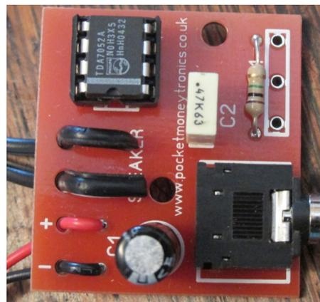
*Above: the optional 1MΩ resistor is located in the top right-hand corner of the PCB. Notice that the 'notch' is on the end of the chip nearest the speaker wires.*
